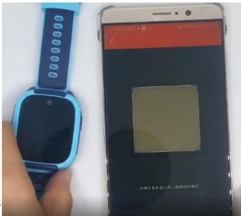
**Step3**, Press and hold the button on the right side of the watch for 3 seconds to turn on the watch. Do not forget open wifi or 4G/3G/2G
